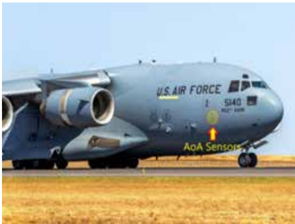
Fig. 2 Pivoted vane type sensor accessed, Source: - Dreamtime
